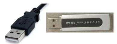
USB connectors have two open square holes on one side and two square holes with plastic below them on the other side. On most computers, you'll plug USB connectors in with the open square holes on the top.
